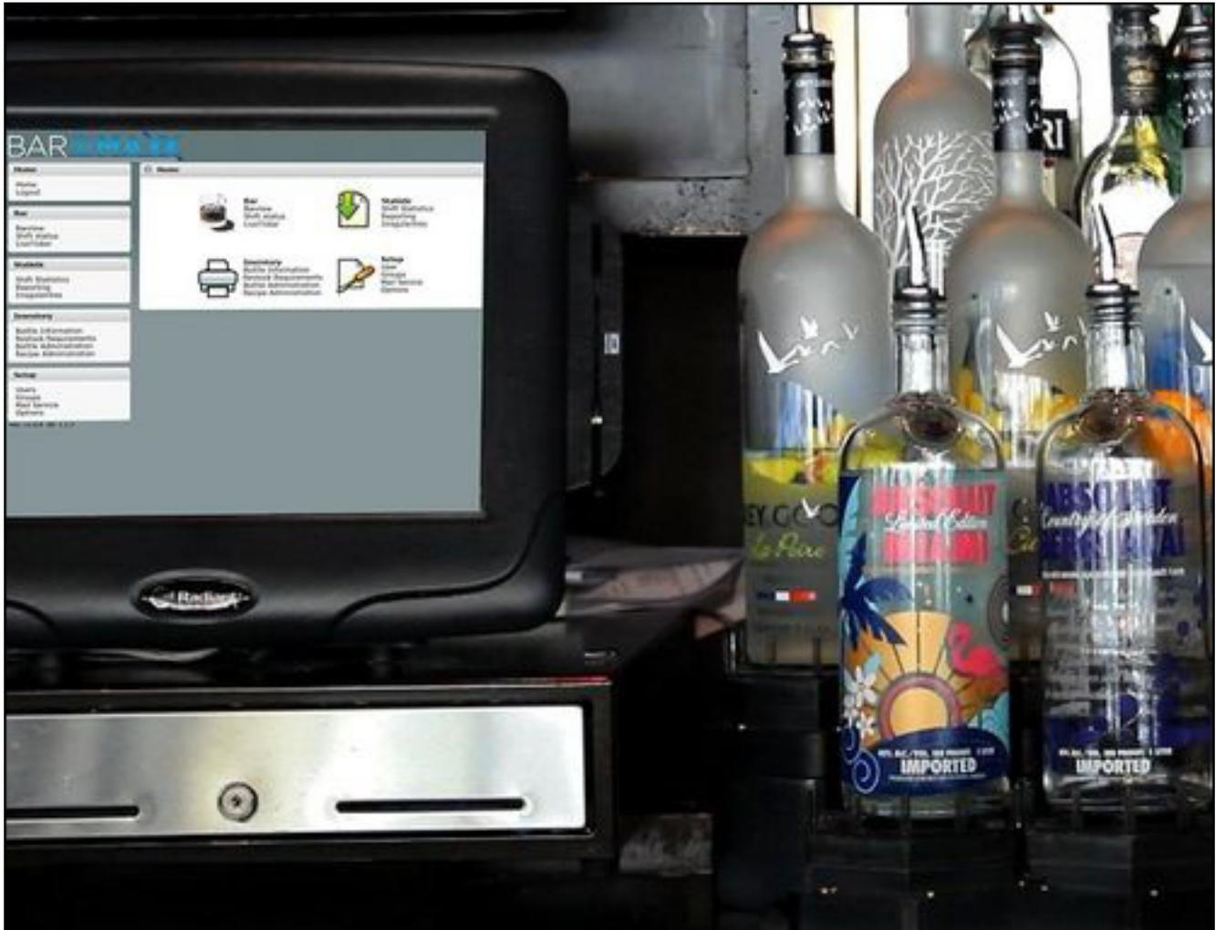
*With the BarMaxx system, an RFID tag is affixed to the bottom of each liquor bottle, which—between pours—is placed on an electronic scale fitted with an RFID reader antenna.*
